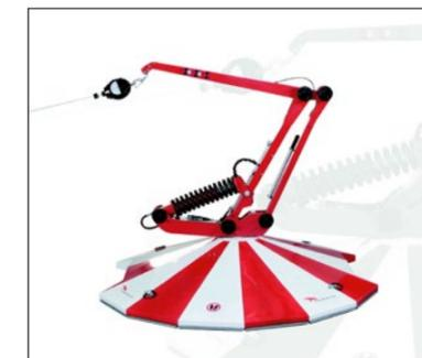
As soon as the permissible payload is exceeded, the safety unit trips: the extension arm retracts and draws the anchor point for the safety harness closer.
