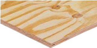
DokaPly BBOES is an economy panel best used in low re-use applications. It has a B face on both sides, which are oiled and the edges are sealed.
