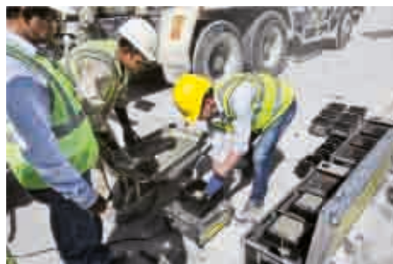
▲ The calibration is made by casting six cubes, measuring their temperature development and testing their compressive strength at a certain maturity. This leads to a correlation curve between maturity and compressive strength.
