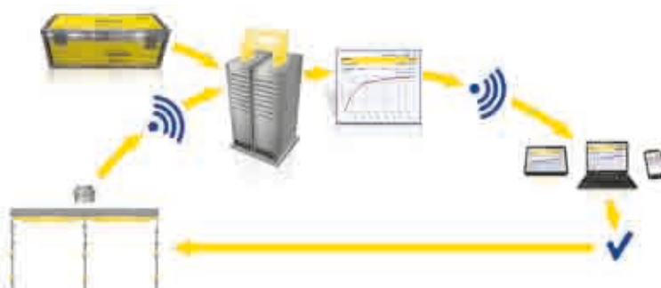
▲ The calibration is made by casting six cubes, measuring their temperature development and testing their compressive strength at a certain maturity. This leads to a correlation curve between maturity and compressive strength.
