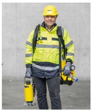
The carrying handle and shoulder strap ensure ergonomic repositioning of hydraulic cylinder and battery hydraulic unit.
