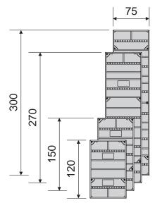
Frami universal panels are available in widths of 75 cm and 90 cm and in panel heights of 120 cm, 150 cm, 270 cm and 300 cm, for column cross-sections of up to 80 cm x 80 cm, in a 5 cm grid.
