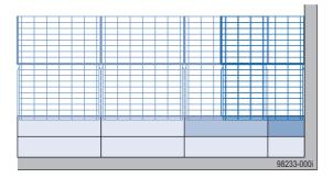
Continue laying formwork sheets and infill sheets in the closure zone in the same way.
