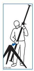
With the prop upright, use the adjusting nut for precision adjustment.
