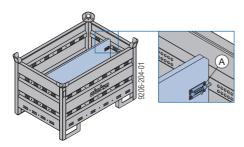
A Slide-bolt for fixing the partition
