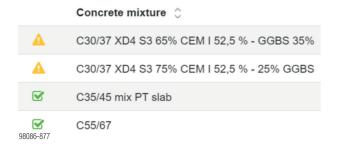
Yellow symbol ... Validation necessary Green symbol ... Calibration curve has been validated Red symbol ... Validation failed, re-validation / re-calibration necessary
