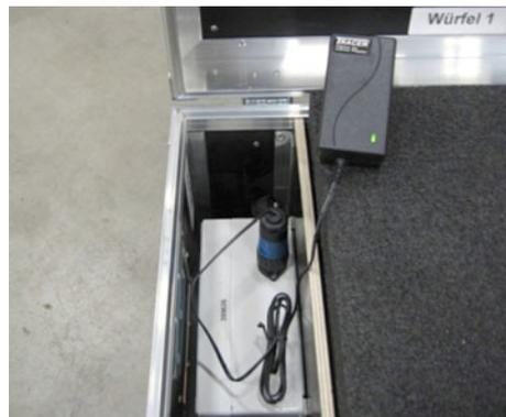
You can make a function test using the power adapter supplied with the box. The green light on the power adapter indicates that the box is fully charged.
