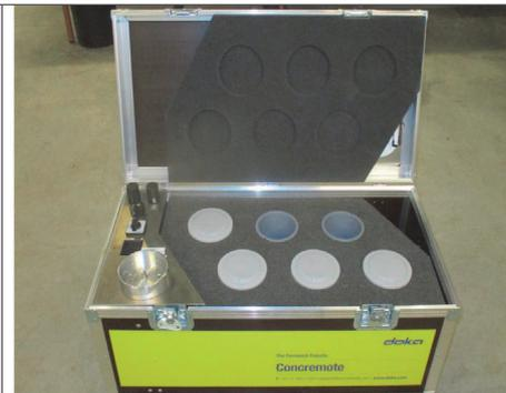
Concremote calibration-box cylinder 2.0 E
