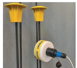
**A** Concremote-Kabelsensor 2.0
