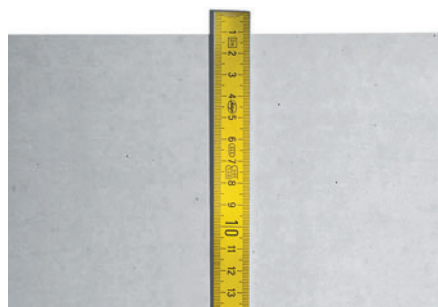
Quantity of release agent applied 10 g/m 2
