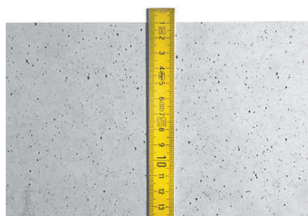
Quantity of release agent applied 30 g/m 2
