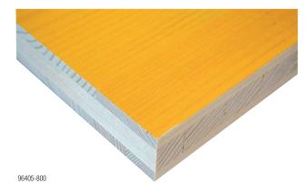
The Doka formwork sheet FF20 is a 3-ply solidwood sheet with urea-melamine resin coating on both sides, for use in wall formwork systems.
