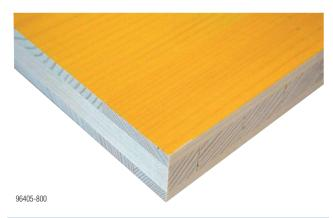
The Doka formwork sheet FF20 is a three-ply solid-wood sheet with urea-melamine resin coating on both sides to Austrian standard ÖNORM B 3023, for use in wall formwork systems.
