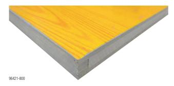
The Formwork sheet 3S top is a high-grade threeply solid-wood sheet with urea-melamine resin coating on both sides to Austrian standard ÖNORM B 3023 and an extra varnish sealant for increased abrasion resistance and reduced texturing and cracking.
