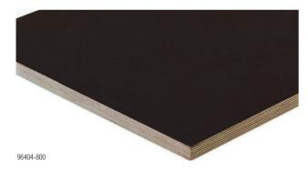
The Dokaplex formwork sheet is a high-grade birchwood-veneer plywood sheet with film coating on both sides, for horizontal and vertical formwork applications.
