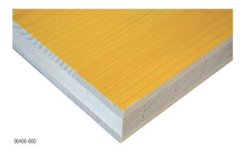
The Doka formwork sheet 3-SO is a high-grade three-ply solid-wood sheet with urea-melamine resin coating on both sides to Austrian standard ÖNORM B 3023, for horizontal and vertical formwork applications.
