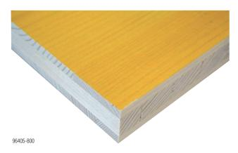
The Doka formwork sheet FF20 is a three-ply solid-wood sheet with urea-melamine resin coating on both sides to Austrian standard ÖNORM B 3023, for use in wall formwork systems.
