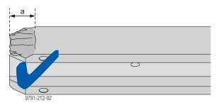
Damage to the plastic cap has no effect on loadbearing capacity, but beams evincing damage of this kind do not necessarily meet the quality criteria for Doka rental formwork.
