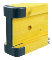
The timber formwork beam H20 pro is a solid-web beam to EN 13377 with high-quality polyurethane end reinforcement for protection against splintering and moisture.
