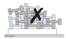
➤ Always stack Beams H20 N "sorted by web thickness", in other words do not put beams of different web thickness in the same row of beams.
