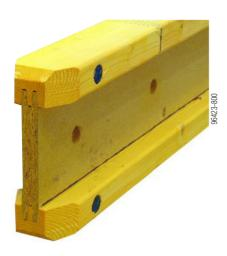
Timber formwork beam H20 eco is a sold-web beam in accordance with EN 13377 with proven end reinforcement in the form of bevelled beam ends and extra plastic rivet in the beam flange.
