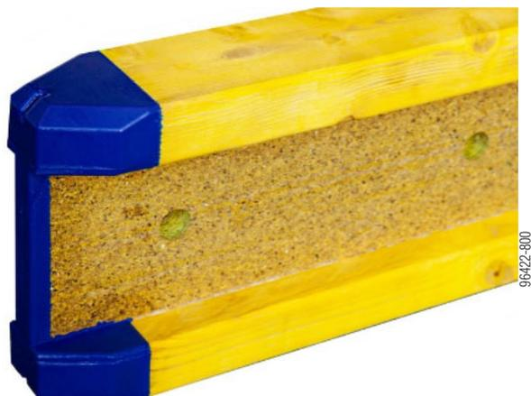
Timber formwork beam H20 top is a solid-web beam in accordance with EN 13377 with innovative polyurethane end reinforcement for increased resistance to mechanical stresses and strains.
