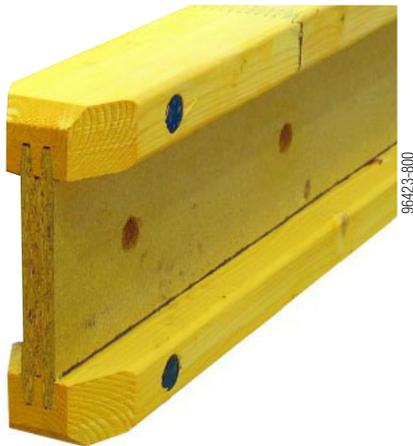
**Timber formwork beam H20 eco is a solid-web beam in accordance with EN 13377 with proven end reinforcement in the form of bevelled beam ends and extra plastic rivet in the beam flange.**
