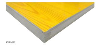
The Formwork sheet 3S top is a high-grade threeply solid-wood sheet with urea-melamine resin coating on both sides to Austrian standard ÖNORM B 3023 and an extra varnish sealant for increased abrasion resistance and reduced texturing and cracking.
