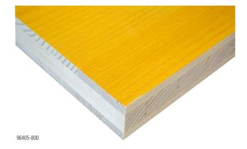
The Doka formwork sheet FF20 is a three-ply solid-wood sheet with urea-melamine resin coating on both sides to Austrian standard ÖNORM B 3023, for use in wall formwork systems.
