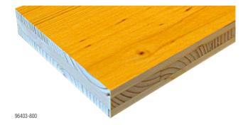
The Doka formwork sheet 3-S plus is a high-grade three-ply solid-wood sheet with urea-melamine resin coating on both sides to Austrian standard ÖNORM B 3023 and an extra varnish sealant on one side for increased abrasion resistance and reduced texturing and cracking.
