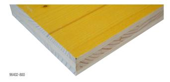
The Formwork sheet 3S basic is a three-ply solidwood sheet with urea-melamine resin coating on both sides to Austrian standard ÖNORM B 3023 in the mid-level quality sector for many different uses on construction sites.
