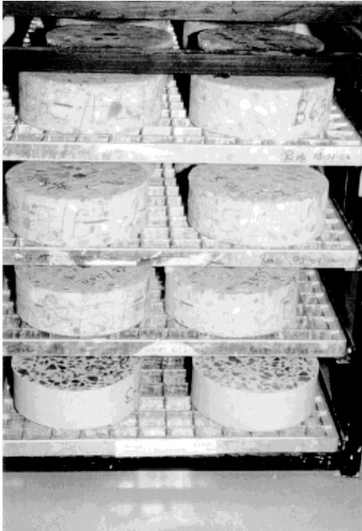
Fig 9: Storage arrangements for the gas-permeability test specimens at 20 °C and 65 % rel. humidity from the 70 th day (end of 1 st test series) until the 210 th day (beginning of 2 nd series of tests).
