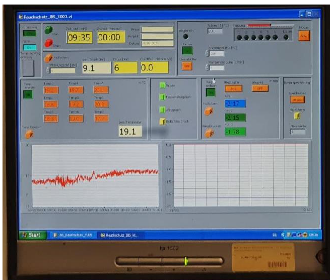
Fig. 14: Readings at pressure of 6 pascals => 0 pressure loss = no air leakage at the form-tie points
