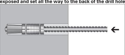
Screw the tie rod into the spreader cone and insert it right down to the back of the bore-hole.
