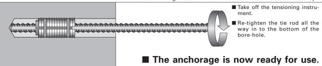
N.B.: After work is completed, the tie rod can be retrieved for re-use, while the spreader unit stays in the bore-hole.
