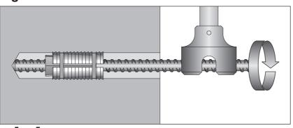
■ Turn the tie rod with the tie rod spanner - the spreading segments now press hard into the walls of the borehole.
