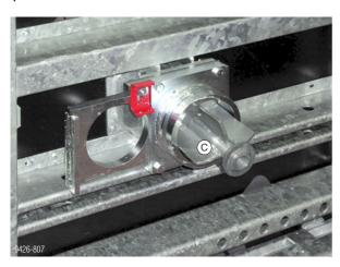
➤ Use the lever coupling to mount the Framax hose to panel coupler SCC to the Framax Xlife universal panel SCC, and turn the spindle to screw the locking part in as far as the slide valve.
