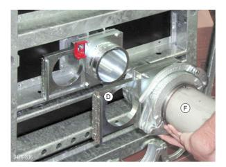
Clean the panel closure tool and insert the locking part.
