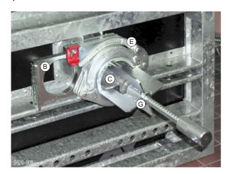
➤ Lift the securing latch and open the slide valve. Screw in the locking part with the Framax hose to panel coupler SCC, as far as it will go.
