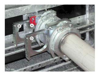
➤ Undo the lever coupling between the slide valve and the panel closure tool.
