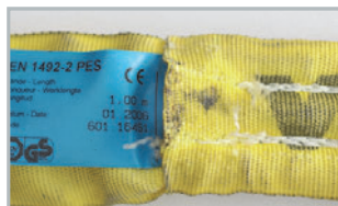
Torn seams in the sheathing
