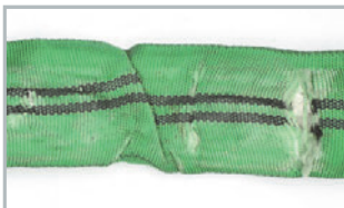
Damage to the sheathing due to abrasion or cuts - if the core is visible, the round sling must be taken out of service immediately!
