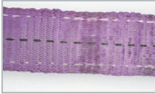
Severe distortion or melting of threads due to heat (shiny surface and/or hardening of the webbing).
