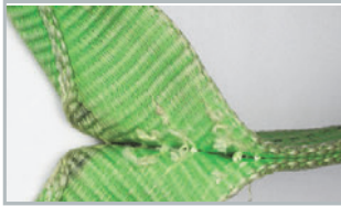
Damage to load-bearing seams
