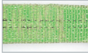
Damage to the fabric caused by abrasion or cutting
