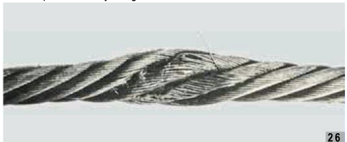
Wire rope flattened by being driven over
