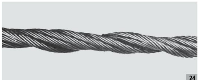
Necking as a result of a destroyed rope core
