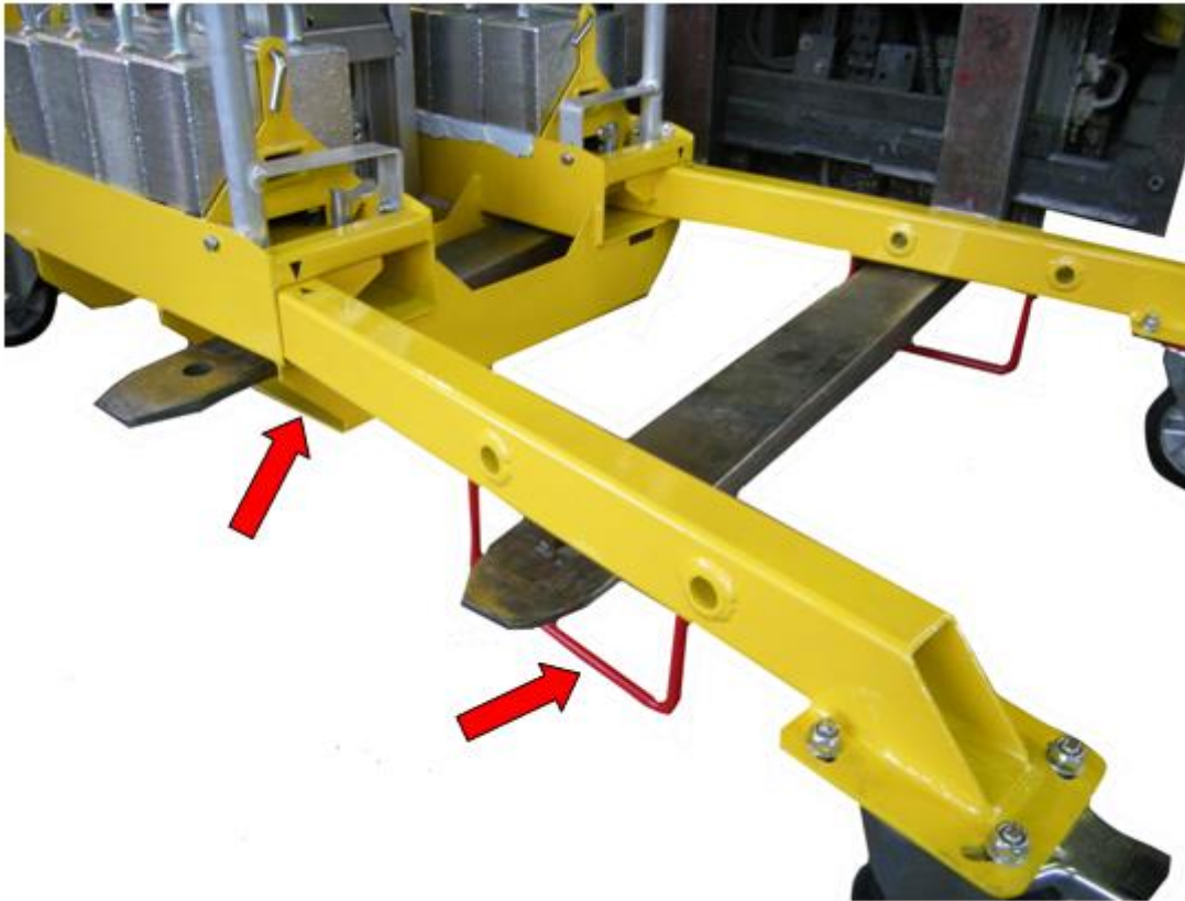
Fig. 38 Supports for forklift transport
