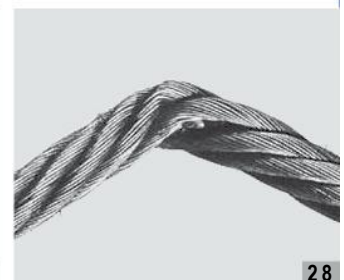
Kink caused by mechanical damage
