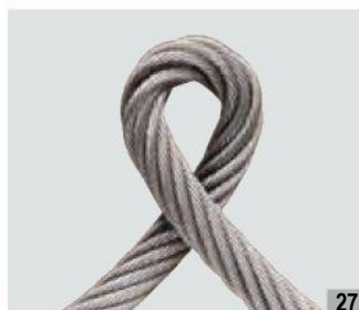
Kink caused by Pinching a loop
