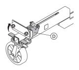
➤ Pull out the wheel as far as it will go. The Safety clip must snap into place.
